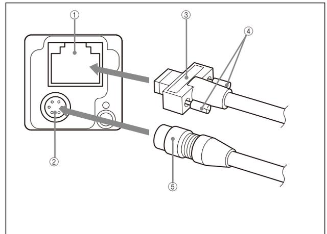
Connect the camera cable to the DC IN connector and connect the LAN cable to the RJ45 connector respectively. If you use a camera module interface board or a hub that supports PoE, you can operate the camera even if you do not connect the camera cable to the DC IN connector. When you connect the LAN cable with fastening screws, turn the two screws on the connector to secure the cable tightly.
