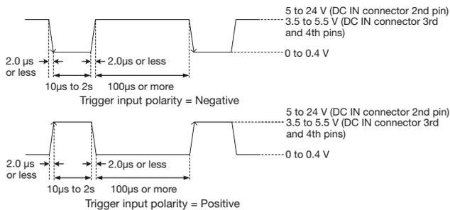
When inputting a trigger signal to the camera using the DC-700/CE, use DC 5 V or less at the logical high level.
