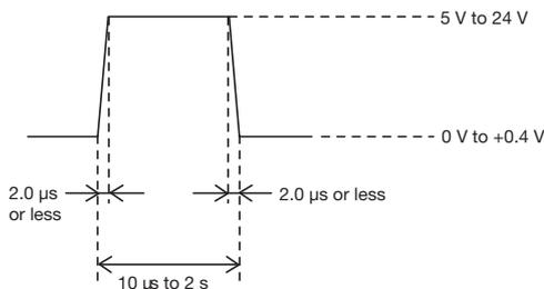
Trigger input polarity = Negative
