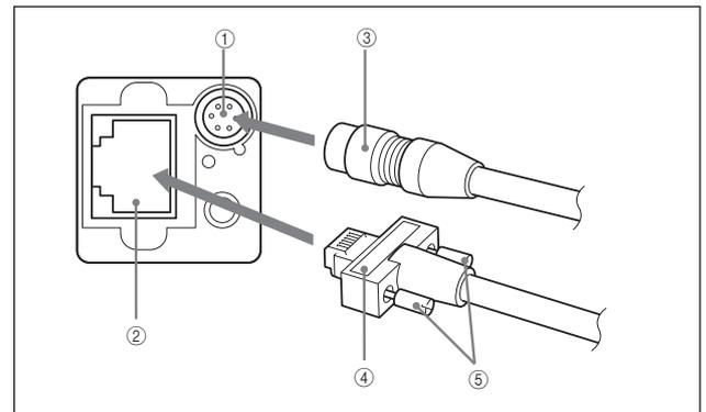
Connect the camera cable to the DC IN connector and connect the LAN cable to the RJ45 connector respectively. If you use a camera module interface board or a hub with support for PoE, you can operate the camera even if you do not connect the camera cable to the DC IN connector. When you connect the LAN cable with fastening screws, turn the two screws on the connector to secure the cable tightly.
