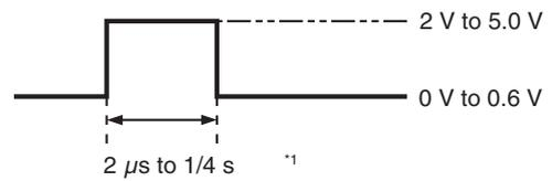
\*1 If you set the trigger pulse with the DIP switches, use the 100  $\mu$ s to 1/4 sec pulse width.
