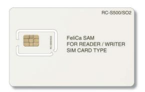
RC-S500/SO2 is the FeliCa<sup>™</sup> SAM for readers that support AES and DES encryption systems. This product enables various terminals to utilize FeliCa security functions for a wide range of applications. In addition, RC-S500/SO2 supports FeliCa Lite-S card.
