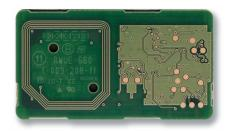
RC-S660/S is a UART-compatible NFC module suitable for incorporating into various embedded devices. This module supports communication with ISO/IEC 14443 Type A / Type B and ISO/IEC 15693 cards and tags, as well as FeliCa™. In addition, as with previous products, the antenna and control have been integrated to maintain a compact size, making it easier to incorporate into a variety of devices.
