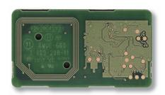
RC-S660/U is an embedded NFC module for PCs, tablets and other consumer electronic devices. This module supports communication with ISO/IEC 14443 Type A / Type B and ISO/IEC 15693 cards and tags, as well as FeliCa™. Its compact design makes it easier to incorporate into a variety of devices.
